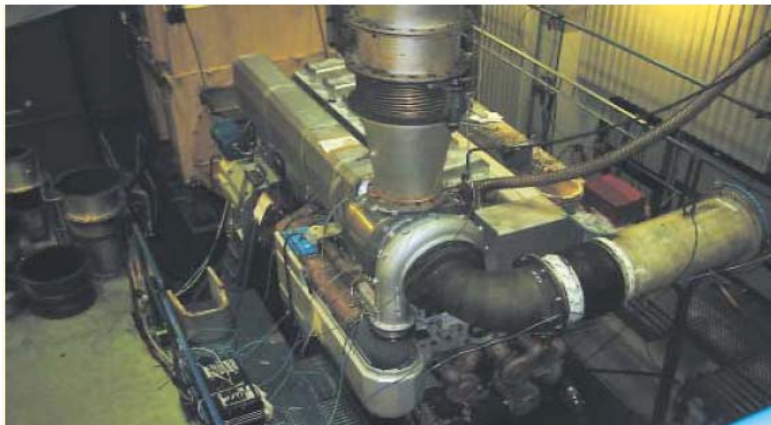
Fig. 5 Wärtsilä 6L32 engine undergoing bio-oil testing.
